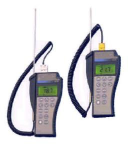
The thermometers-calibrators can simulate temperatures thanks to thermocouples (PJ6521) or resistive probes Pt100 (PJ 6522), and measure these same sensors to calibrate temperature measuring or temperature regulation instruments.
